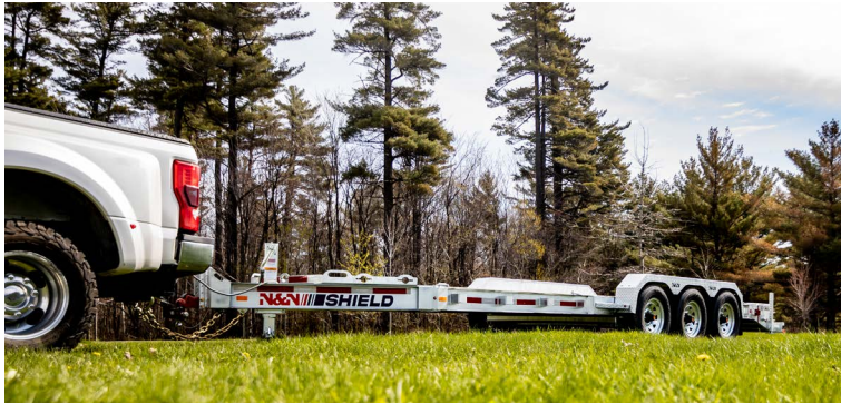
Model shown: 3-foot beavertail drop with flip over ramp
