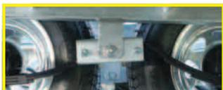
Slipper spring suspensions on our tandem models require less maintenance. Certain N & N models can be greased.
