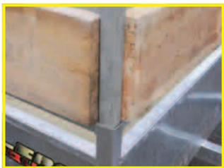
Open corner posts make an easy job of adding additional panels to increase the height of the sides of the trailer.
